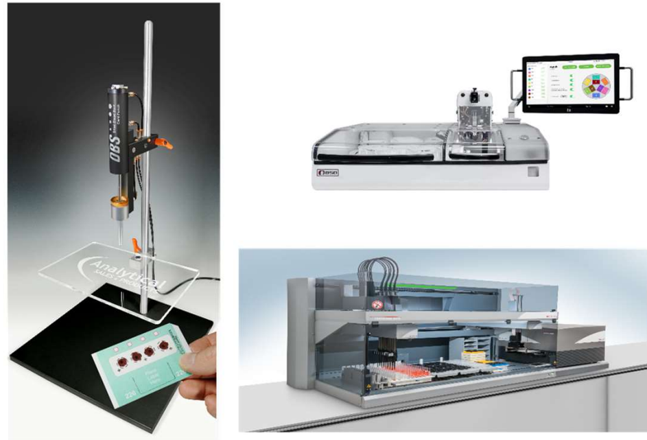
FIGURE 5.1. Commercially available (semi-)automated punching and pipetting instruments. From top-left to bottom-right: the DBS Pneumatic Card Punch (Analytical Sales and Services), the BSD GalaxyA9 (BSD Robotics) and the Freedom EVO Robotic Handler (Tecan). Reproduced with permission of Analytical Sales and Services, BSD Robotics and Tecan.
